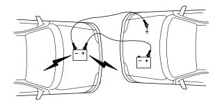
4. Make the final connection of the negative (-) cable to an exposed metal part of the stalled vehicle's engine, away from the battery and the carburetor/fuel injection system.
